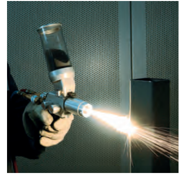
Cold Spray process with UTP COLDmelt™ stainless 18
