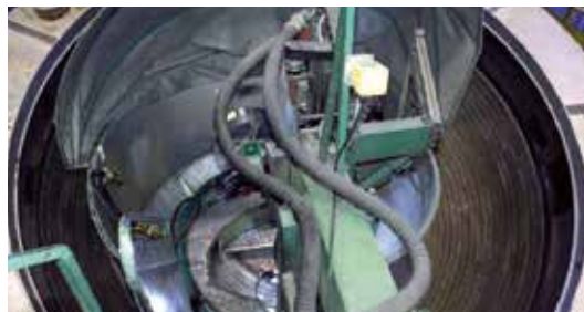
Steam Generator Expansion Tank Soudotape 308 L Q5 + Record 8B308T1 Q5 Soudotape 309 L Q5 + Record 8B308T1 Q5
