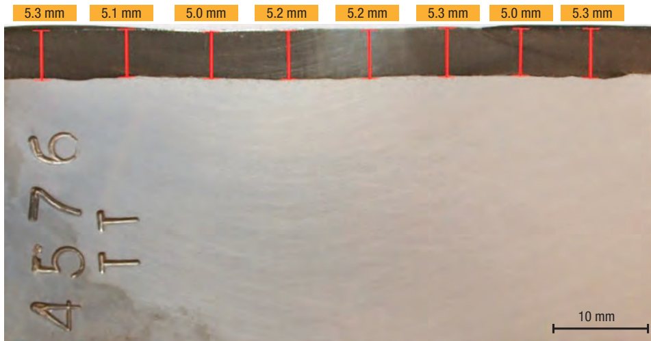
Figure 3: Bead profile of cladding with RECORD EST 625-1 LD, with <7% Fe scenario.
