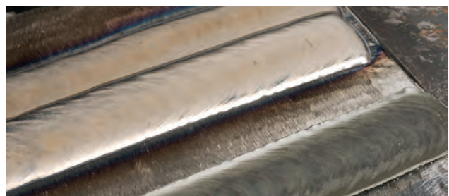
Figure 6: Cladding with RECORD EST 625-1 LD: flat beads, straight edges, no slag adherences.
