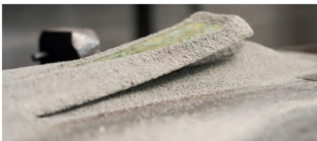
Figure 5: Cladding with RECORD EST 625-1 LD: self-releasing slag.
