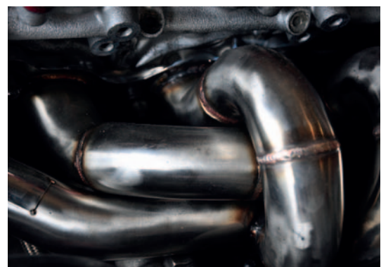
Weld seams on an exhaust manifold
